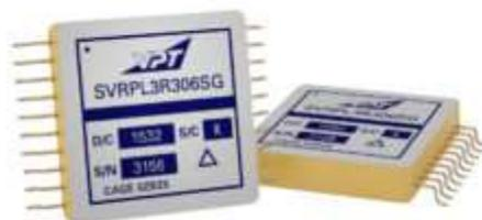
*Figure. The SVRPL3R306SG operates from 3.1-V to 5.5 V input, with an adjustable output from 0.8 to 3.8 V at up to 6 A of output current. It offers highly efficient operation—up to 95%.*
