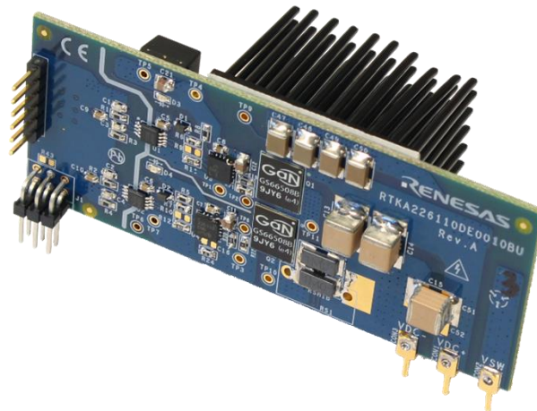
Fig. 1. The GS-EVB-HB-66508B-RN is a 650-V 30-A GaN half-bridge and RAA226110 gate-driver demonstration board. This evaluation kit consists of two GaN Systems GS66508B 650-V GaN E-mode transistors and all necessary circuits including half-bridge gate drivers, isolated power supplies and optional heatsink to form a functional half-bridge power stage. It allows users to easily evaluate the GaN E-modes performance in any half-bridge-based topology, either with the universal motherboard or the users' own system design. The GS-EVB-HB-66516T-RN is similar but contains a 650-V 60-A GaN half-bridge employing two GaN Systems GS66516T GaN E-mode transistors.
