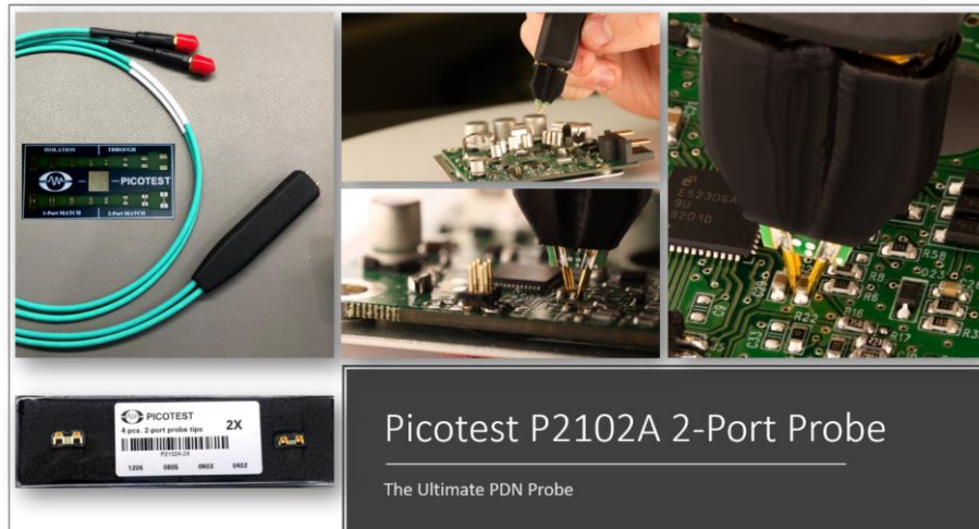
Fig. 1. The P2102A PDN probe enables PDN low and ultra-low impedance measurements for power integrity applications. In the past, performing PDN impedance measurement required soldering of coax or preparing the PCB with RF connectors for measurement. The P2102A is referred to as a "browser" probe for its ability to easily and quickly be moved from point-to-point/rail-to-rail simply by reseating the probe points. The probe can measure submilliohm power rail impedances up to bandwidths of 300 MHz; comes with four swappable heads in sizes that match those of common output capacitors and is available in different attenuations, for measuring across a wide range of voltages.
