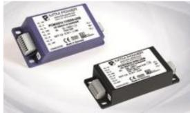
The devices supply up to 2 A per charging port; the charging current between the charger and the charging client is determined by communication lines based on USB specifications. If the communication lines are not connected or there is no communication, the charging client is
