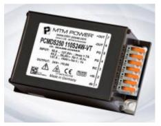
The dc-dc converters are now connected via push-in cage-clamp connectors with lever, which are designed for wire cross sections up to 4  $\rm mm^2$ . Designed for an operating temperature range of -40°C to + 70°C (class TX according to EN 50155) the cooling is guaranteed either by the integrated heatsink (option WK) or by mounting the baseplate on a heat dissipating surface.
