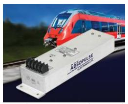
The railway converters offer wide EN50155 dc input ranges of 24 V (14.4 to 34 V), 36 V (22 to 51 V), 48 V (29 to 67 V), 72 V (43 to 101 V), 96 V (58 to 135 V) or 110 V (66 to 154 V). The 200-W units provide outputs of 12 V, 24 V or 48 V. Custom input and output voltages are available on request. Regulation is better than 1% from zero load to full load across all line and load conditions. Efficiency is 80% to 90% depending on input/output configuration.
