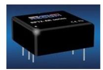
RECOM's RP12-AR dc-dc converter series offers compact 12-W 1-in. x 1-in. modules that operate with 90% efficiency and at temperatures up to +88°C ambient at full load. The converters are designed for railway rolling stock applications, but they are also suitable for non-railway high-voltage battery applications. Their 5:1 dc input voltage range of 36 to 160 V (185 V for 1s) allows for all-in-one solutions for 48-V, 72-V, 96-V and 110-V dc railway systems.
