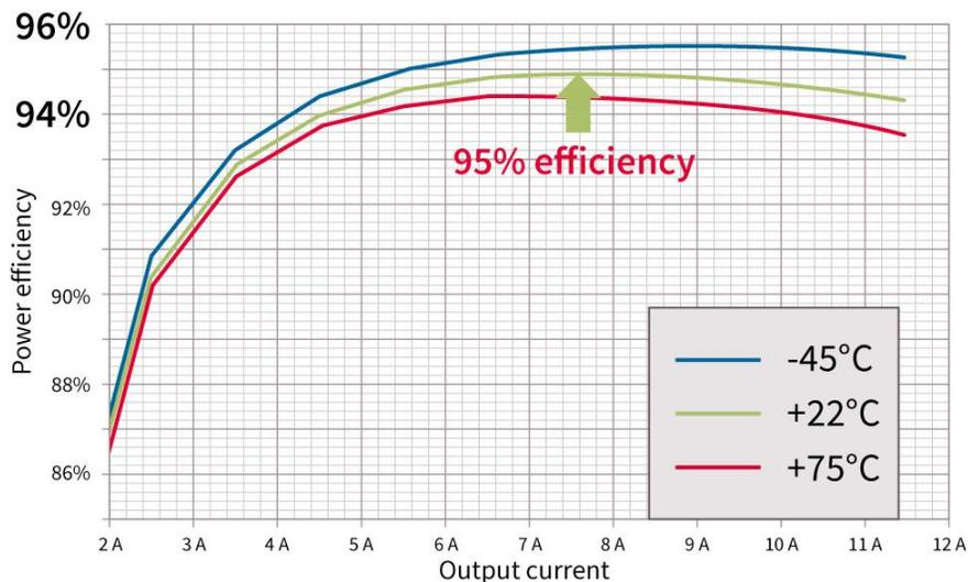
Fig. 7. Measured efficiency vs. load curve (without auxiliary power supply consumption).
