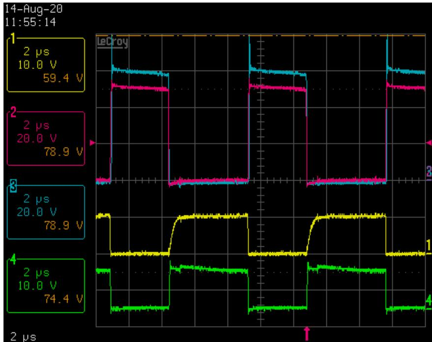
Fig. 4. Gate and drain voltage waveforms across MOSFETs Q4 and Q6, the low-side switches in the full bridge and synchronous rectifier, respectively. Ch 1 = Q4 gate voltage, Ch 2 = Q4 drain voltage, Ch 3 = Q6 drain voltage and Ch 4 = Q6 gate voltage.
