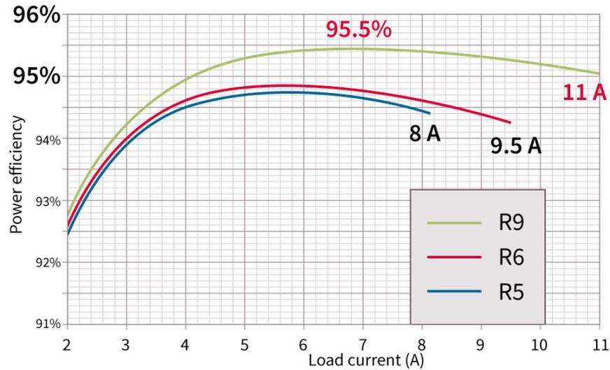
Fig. 6. Modeled efficiency vs. load curve of rad hard dc-dc converter obtained at a 25°C baseplate temperature ( $V_{out} = 24\text{ V}$ ).
