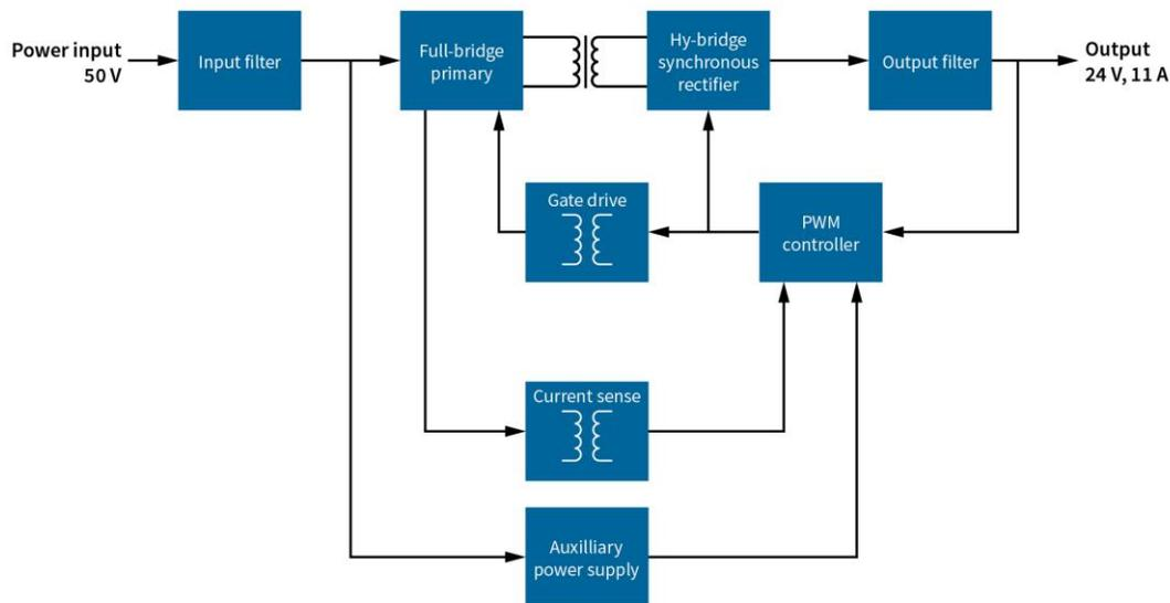
Fig 1. Block diagram of IR HiRel’s rad hard 260-W isolated dc-dc converter.
