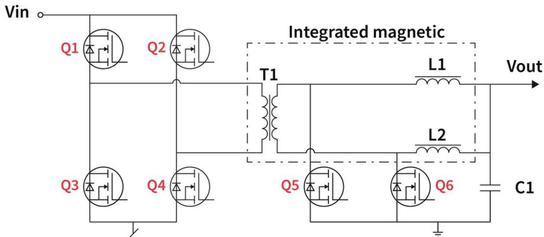
Fig. 2. Simplified power stage schematic.
