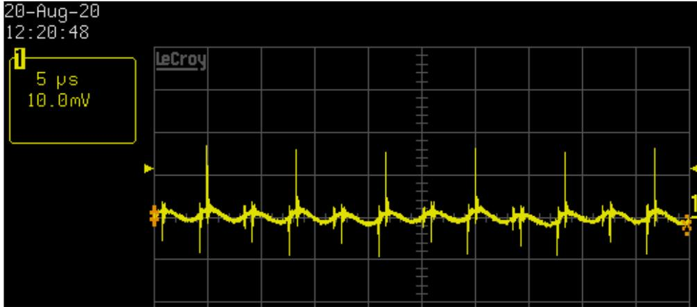
Fig. 5. Output voltage ripple. The asymmetry observed in the waveform of the output voltage ripple is due to the noise from the main transformer being picked up by the measuring probe at the output.
