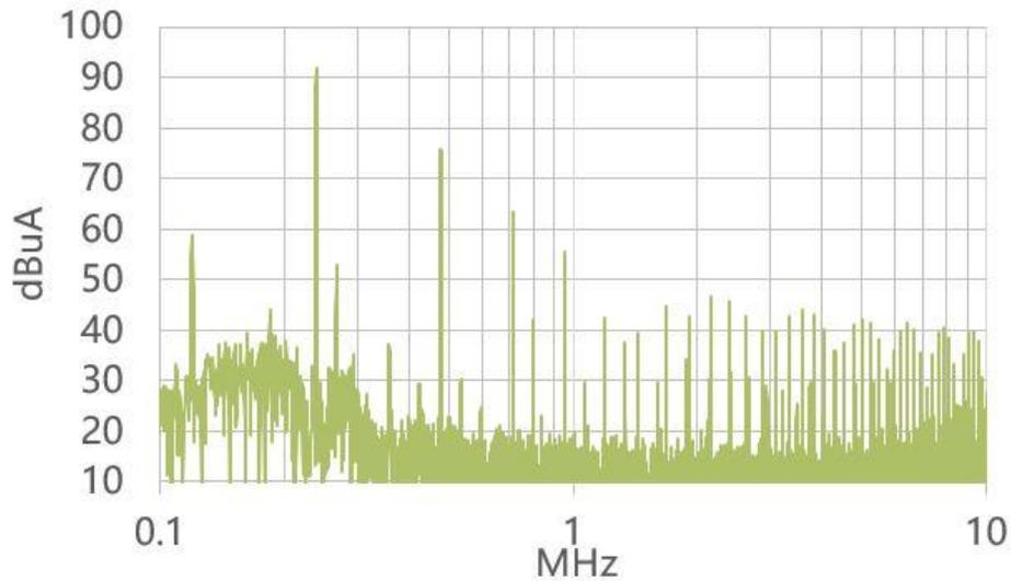
Fig. 3. Conducted EMI at the input of dc-dc converter.
