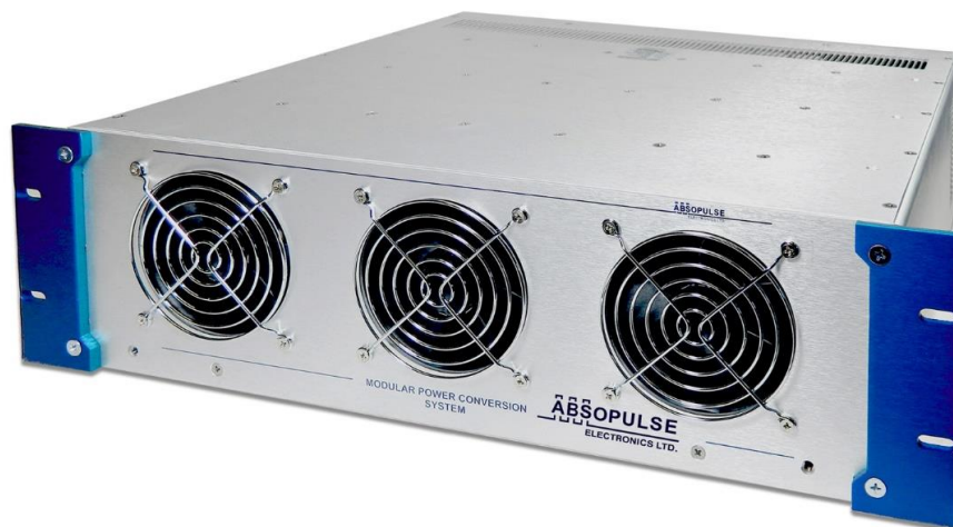
Figure. The PFH 5K-A3P/XX-3U7 series 5-kW ac-dc power supplies with three-phase active PFC-input operate from a three-phase input of 208 Vac (197 to 264-Vac operating range) and deliver any single dc output from 24 V to 400V. A similar version that operates from 400-Vac three-phase sources is also available. The power supplies comply with EN61000-3-2 and EN61000-3-12 directives for low input harmonic distortion. Power factor is better than 0.97 at full load for the entire input range
