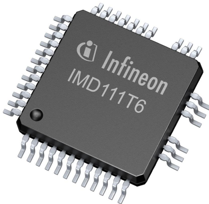
Fig. 1. The IMD110 iMOTION Smart Driver integrates motor controller and a 600-V three-phase gate driver in an LQFP-40 package.
