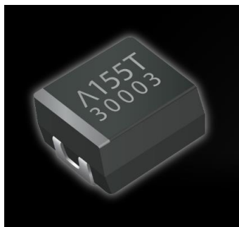
Figure. Now available in five miniature, low-profile case sizes with capacitance and voltage ratings spanning 10 to 470 \mu\text{F} and 2.5 to 50 V, AVX's AEC-Q200-qualified TCQ series capacitors deliver double the operational life required in the AEC-Q200 specification, 2,000 hours at 125^{\circ}\text{C} .
