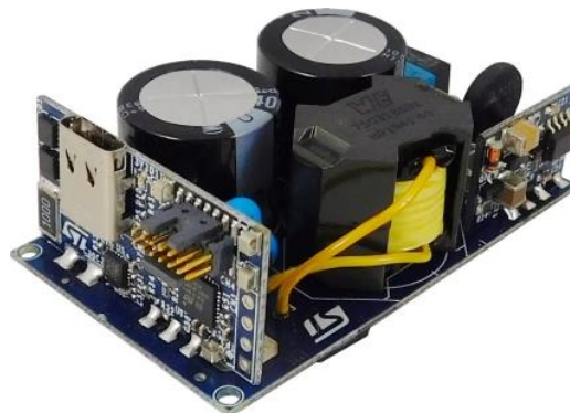
Figure. The STEVAL-USBPD27S 27-W ac-dc adapter reference design works as a USB Power Delivery provider with a single USB Type-C port supporting Programmable Power Supply (PPS) and featuring adaptive synchronous rectification. The reference design accepts a wide range of input voltages and delivers two well regulated fixed PDOs (5 V at 5 A, 9 V at 3 A) and two APDOs (5 V prog at 5 A and 9 V prog at 3 A), finely adjusted to the advertised voltage range (PPS), thus managing the V_{CONN} , as requested by the USB PD specification.
