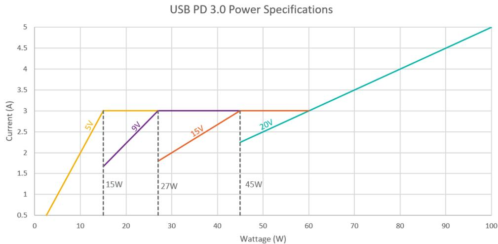
*Fig. 3. USB PD 3.0 voltage and current capabilities.*
