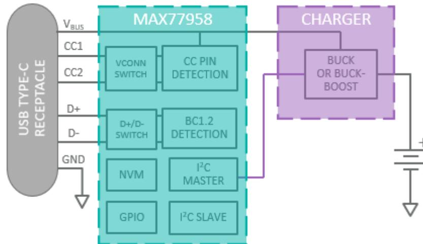
Fig. 5. USB Type-C v1.3 and PD 3.0-compliant standalone PD controller.
