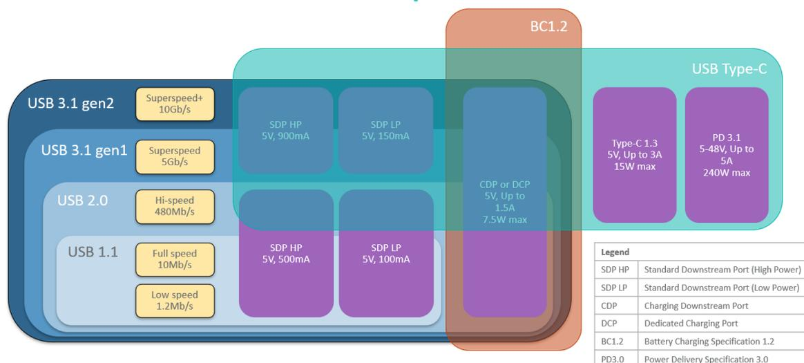
Fig. 2. Power capabilities of each USB specification.
