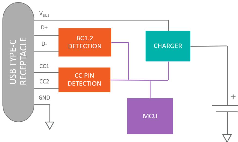
Fig. 4. USB PD design block diagram.
