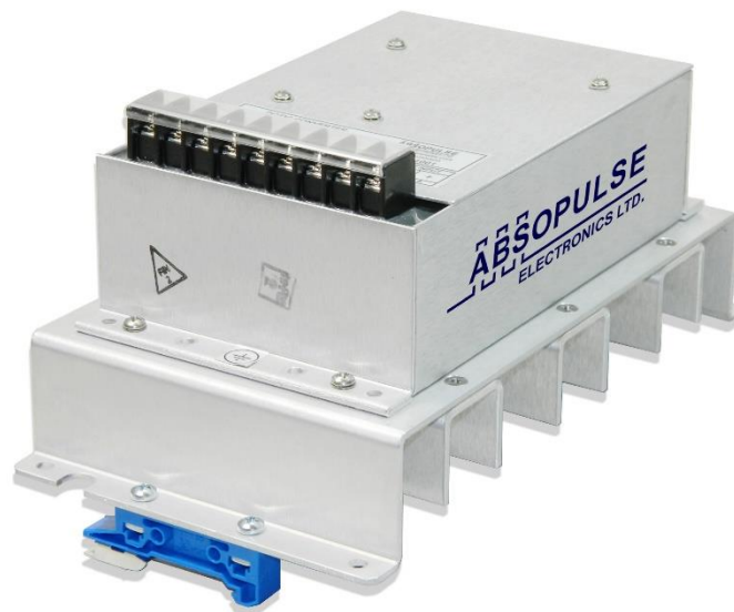
Figure. A member of the PDC 250-HSA-P59 series, this fully encapsulated, industrial-quality, dc-dc converter uses field-proven technology to generate the required output power. It is a mature product with a track-record in numerous applications. The converter is entirely potted with a thermally conductive MIL-grade silicon rubber compound to provide immunity to shock, vibration and humidity. Encapsulation ensures heat dissipation throughout the module. Convection cooling is achieved by installing the unit on a heatsink assembly block which is specifically designed for the unit.
