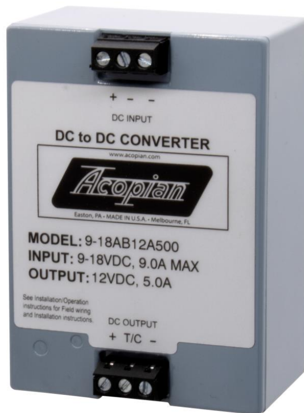
Figure. These mini-encapsulated, single-output, wide-input dc-dc converters with touch-safe terminal blocks have the versatility to be used in a broad range of applications including those in automotive, ATE, OEM, military and industrial/manufacturing. Dc inputs range from 9 V to 18 V, while dc outputs range from 3.3 V to 48 V and up to 7 A. Threaded mounting holes permit them to be mounted to a chassis, cabinet wall or bracket, or they may be used on a test bench or tabletop.
