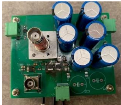
Fig. 3. Double-pulse test board for the BUK7S1R0-40H.
