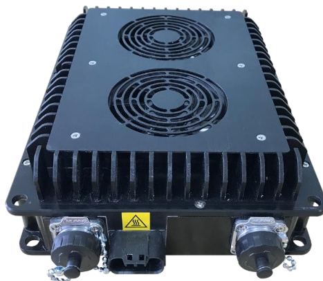
Figure. The EVC-2400 series supports a constant current, constant voltage and constant power charging. The charging current and voltage are controlled through CAN communication. The charger has been designed for a variety of applications including the on-board charging of electric vehicles and the battery systems contained within them.
