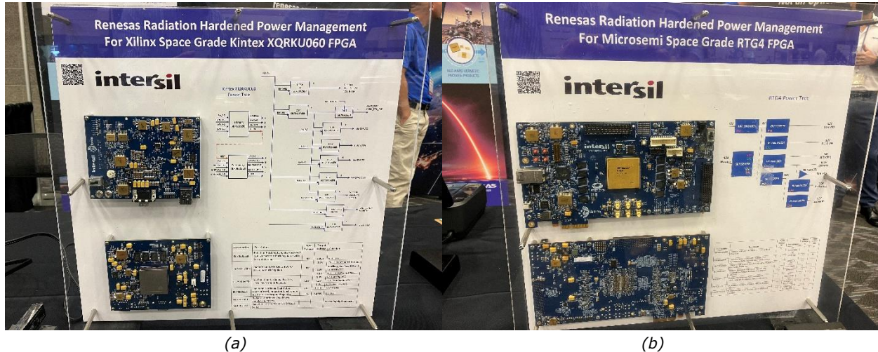
Fig. 1. Renesas's rad-hard power management reference designs for the Xilinx Kintex XQRKU060 FPGA (a) and the Microsemi RTG4 FPGA (b) include devices such as the ISL70321SEH power supply sequencer, ISL70001ASEH synchronous buck regulator, ISL75051ASEH LDO, the ISL770005SEH dual-output POL, sync buck and LDO and the ISL70062SEH load switch—among others.
