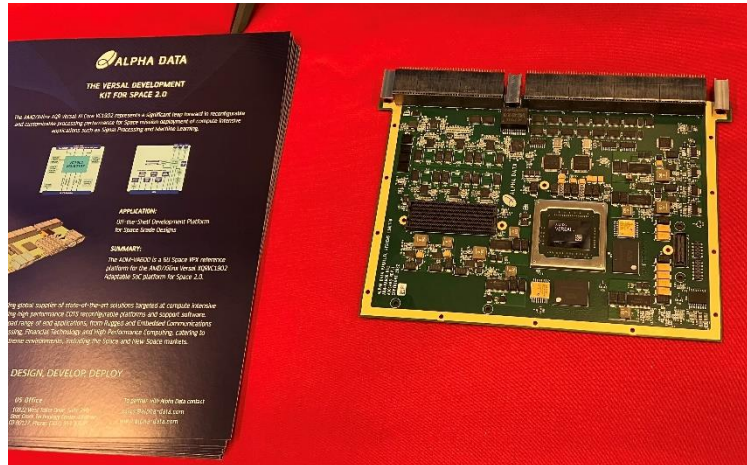
Fig. 7. The Versal development platform for the Versal space-grade (radiation-tolerant) FPGA from Xilinx is described as a flight-ready board. Alpha Data plans to begin offering this board for sale by the end of the year.
