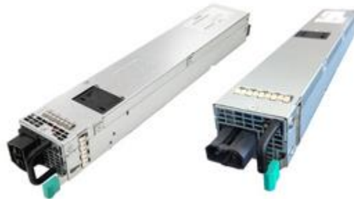
Figure. The D1U54T-M-2500-12-HxxC is a series of 2500-W 54.5-mm wide highly efficient ac and HVDC input front end power modules that provide a 12-Vdc main output and a standby output. The low-profile units achieve >58 W/in 3 and provide active current sharing capability, a multifunction status LED, hardware logic signals, and PMBus digital communications. This power module is well suited for delivering reliable power to servers, workstations, storage systems and other 12-V distributed power architectures. The D1U54-D-2500-12-HxxC is a series of highly efficient low-voltage dc (LVDC) input front end power supplies with similar features.
