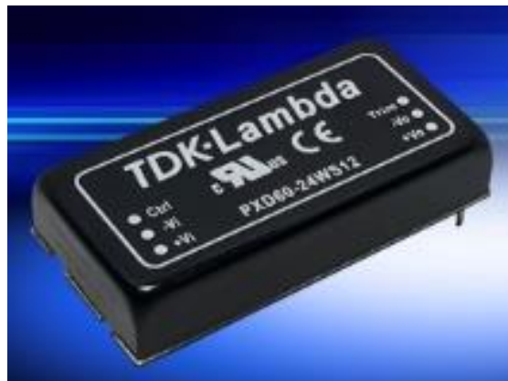
Figure. Packaged in the industry-standard 2-in. x 1-in. footprint, the TDK-Lambda brand PXD40 and PXD60 series 40-W and 60-W dc-dc converters can operate over a wide 4:1 input range, accepting either a 9- to 36-Vdc or 18- to 75-Vdc input, and generate single outputs from 3.3 to 48 Vdc or dual outputs of \pm 12 , \pm 15 and \pm 24 Vdc. Six-sided shielding reduces radiated emissions and simplifies system compliance.
