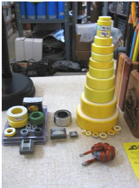
Fig. 1. Iron-powder Micrometals toroid cores shown in the stack and on the left are made of materials 26 (the yellow and white cores) and 52 (the lone green core), which are often optimum for inductor applications when the highest performance is not critical. Higher magnetic performance at higher cost is achieved by the wound gray NiFeMo Magnetics Inc. core in front of the Fe-pwd core tower. The dark gray EE cores with bobbins to the left of the tower are also Micrometals Fe-pwd cores on the Innovatia list.
