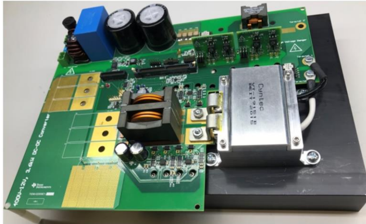
Fig. 6. Photo of the bidirectional dc-dc regulator implementation.
