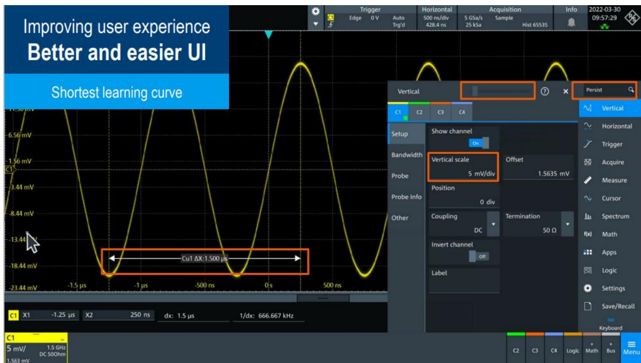
Fig. 3. The scopes incorporate several features that enhance their usability including box design for better touchability, a cursor that displays dynamic values, a search-in menu, a toolbar to make workflows quick and easy and R&S SmartGrid functionality.
