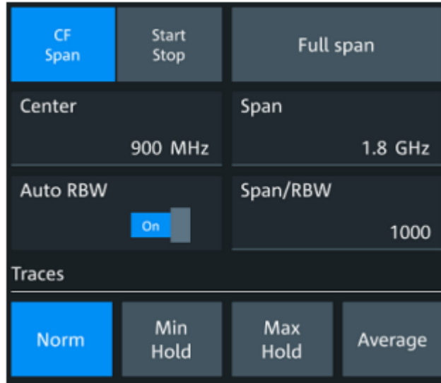
Fig. 2. For spectrum analysis, the MXO 4 series offers independent span/RBW control vs time base and automatic peak list and max/min-hold measurement.
