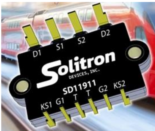
Figure. The SD11911 and SD11912 1200-V SiC power modules house two independent, high-current MOSFETs in a robust 37-mm x 25-mm x 9-mm package that is said to be a fraction of the size and weight of competing modules.
