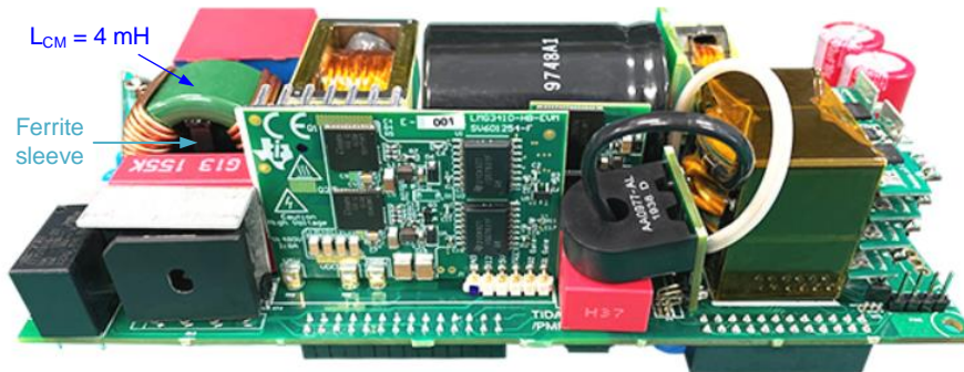
Fig. 13. A totem-pole power factor correction ac-dc and half-bridge LLC dc-dc regulator include a single-phase EMI filter with ferrite choke.
