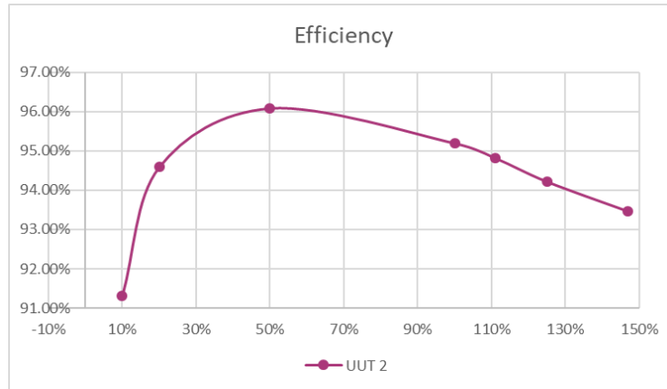
Fig. 8. Even without heatsinks, the SMPS' efficiency remains high while operating up to 150% of nominal load.
