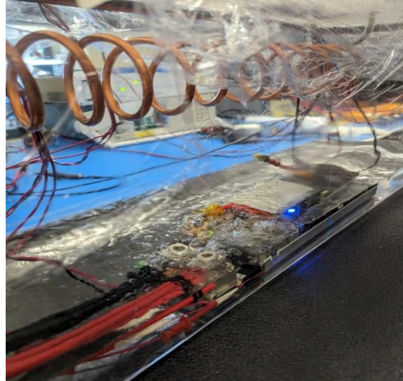
Fig. 4. Experiment with an immersed 2.7-kW PSU.
