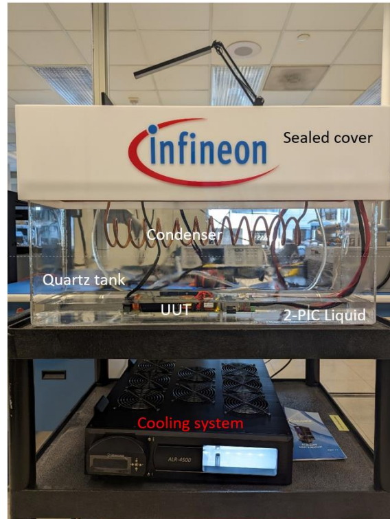
Fig. 3. The components of this liquid cooling experiment included a quartz tank, a condenser, 2-PIC liquid and the unit under test (UUT).
