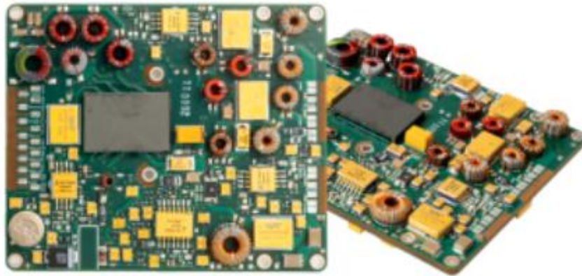
Fig.1. The SLNP17-100CQ is an extremely low noise, quad-output 17 -W dc-dc converter designed for RF space applications. It was built to withstand the harsh radiation environments encountered in demanding commercial, scientific, and military space systems. Performance is guaranteed through the use of radiation lot acceptance tested (RLAT) components. Thanks to a multi-stage approach, the SLNP achieves an exceptional rejection of noise for both conducted emissions (see Fig. 2) and conducted susceptibility.
