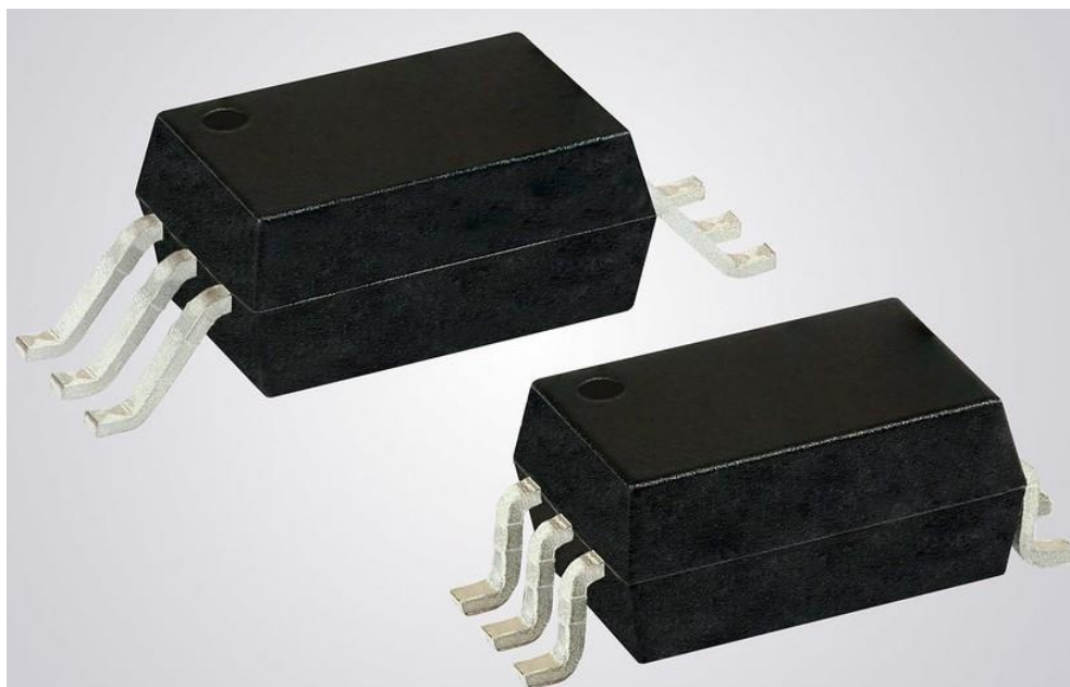
Figure. Consisting of an AlGaAs LED optically coupled to an integrated circuit with a power output stage, the optocouplers are intended for solar inverters and microinverters, ac and brushless dc industrial motor control inverters, and inverter stages for ac-dc conversion in UPS. The devices are well suited for directly driving IGBTs with ratings up to 1200 V and 100 A.
