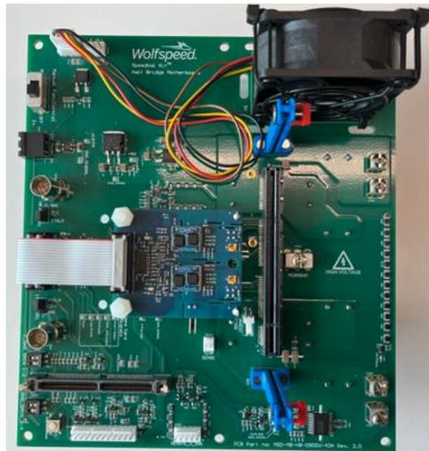
*Fig. 4. The AHV85311 isolated gate driver is combined with Wolfspeed’s SpeedVal kit in a design that delivers up to 10 kA. The gate driver is mounted on the blue daughter card.*
