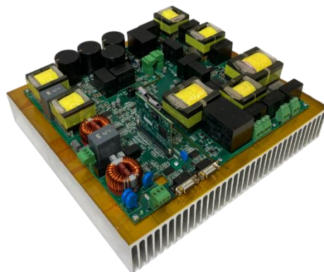
Fig. 1. A 10-kW single-phase reference design based on GaN.
