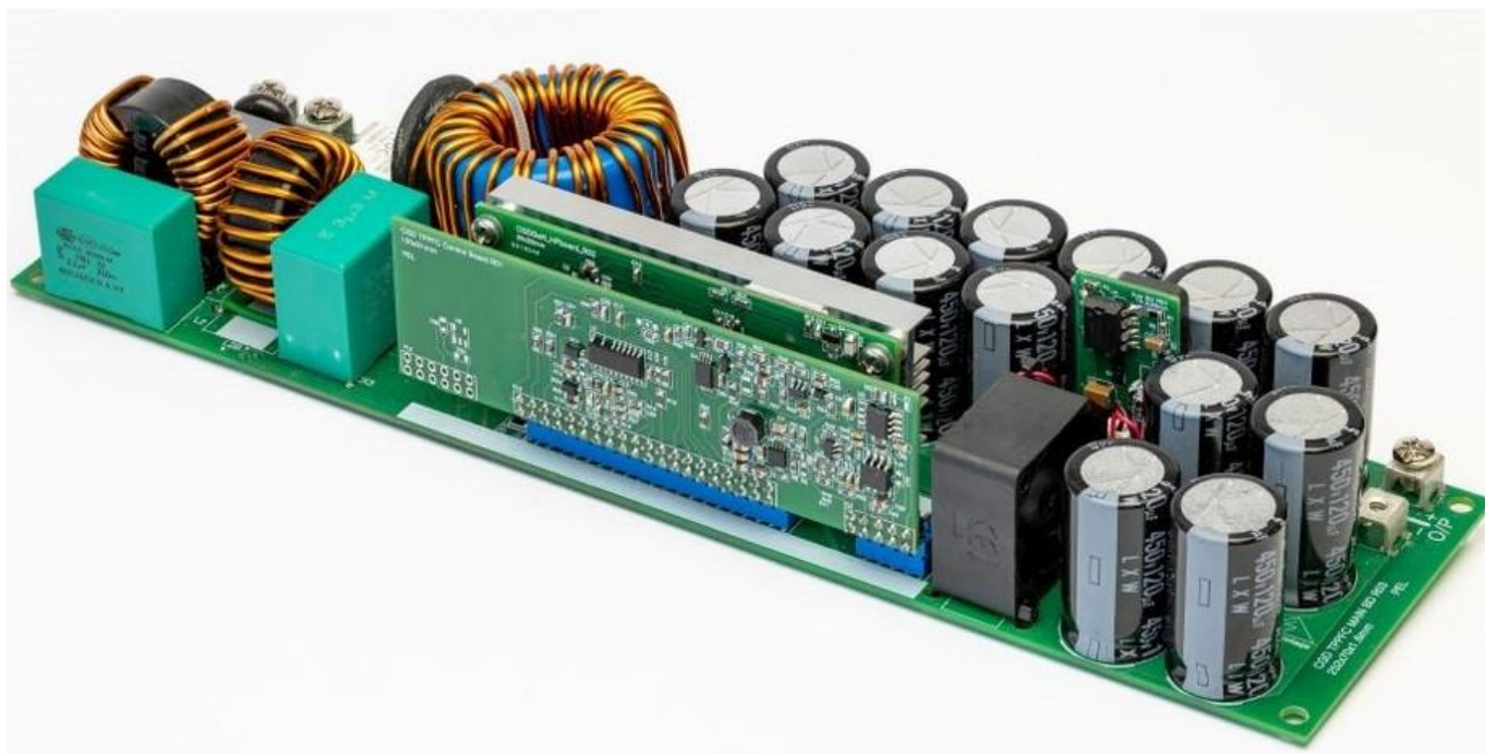
Figure. The CGD-ASY-EVB030FA-01 is a 3-kW totem-pole PFC evaluation board engineered to deliver exceptional efficiency, meeting 80+ Titanium standards when paired with a downstream dc-dc converter. It is optimized for high-power density applications, including high-performance computing, industrial systems, and data servers.
