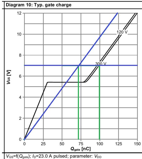
Fig. 6. Extrapolation of Qm1 and Qm2 from the gate-charge characteristic.
