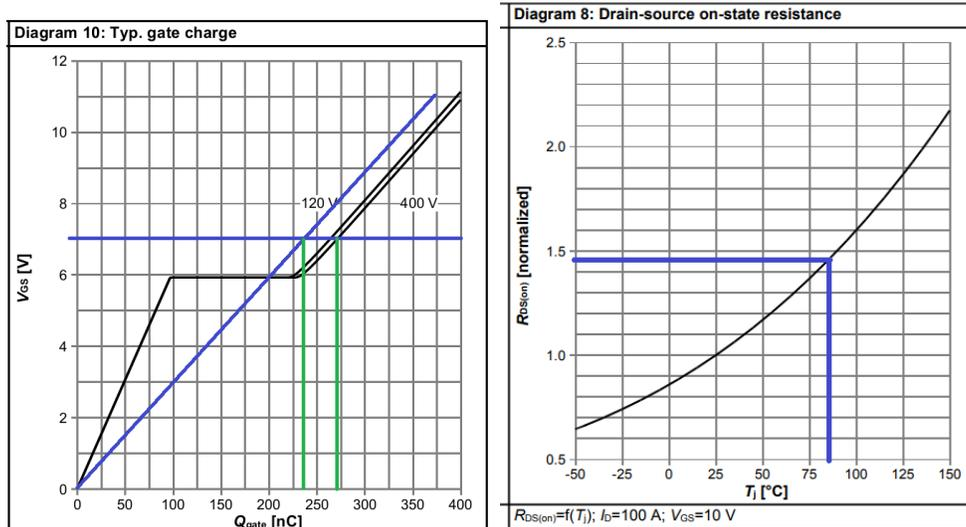
Fig. 8.  $R_{DS(on)}$  and  $Q_g$  values for IPDQ 60R007CM8.
