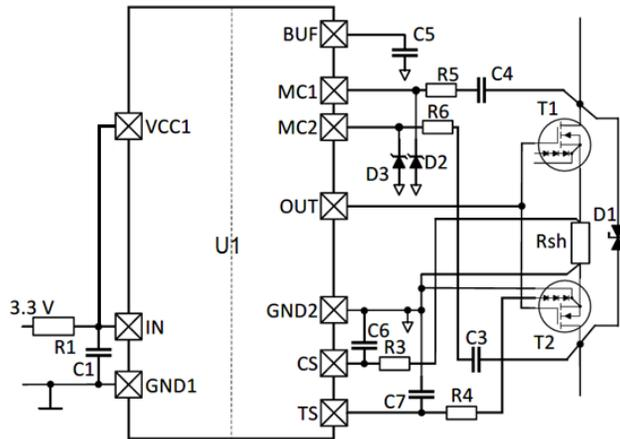
Fig.7 (again). SSR application schematic.
