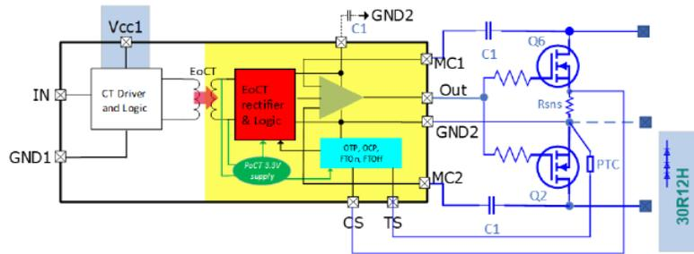
Fig. 1. Highly integrated solid-state isolators, such as the iSSI30R11H/12H, easily drive MOSFETs or IGBTs, and do not require an isolated bias supply.
