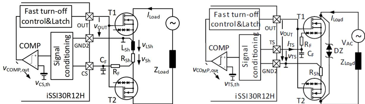
Figs. 2 and 3 (again). Circuitry to implement overcurrent protection using an iSSI30R12H isolator driver. (left) The iSSI30R12H's overtemperature protection triggers within 500 ns (right).
