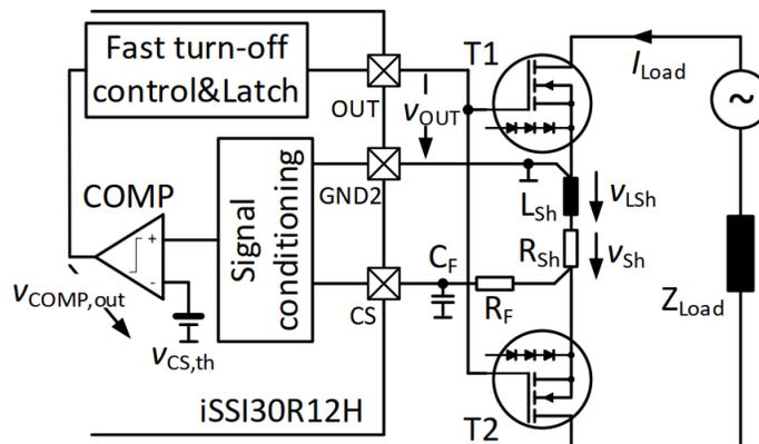
Fig. 2. Circuitry to implement overcurrent protection using an iSSI30R12H isolator driver.
