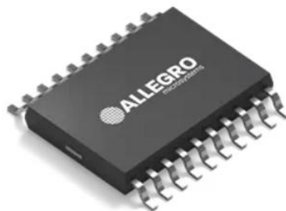
Fig. 3. The A89347 40-V three-phase sensorless BLDC fan driver IC is said to offer whisper-quiet operation in automotive applications such as seat cooling fans, HVAC blowers, and other thermal management systems. The device includes closed-loop speed control with sinusoidal drive to minimize vibration and noise, and integrates EEPROM customization to enable optimized performance and efficiency.
