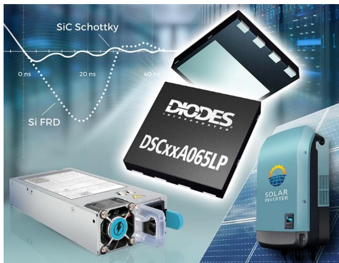
Figure. The compact and low-profile T-DFN8080-4 surface mount package, which measures typ. 8 mm x 8 mm x 1 mm, incorporates a large underside heat pad that reduces thermal resistance. Requiring less board space and providing a larger heat pad, the T-DFN8080-4 is well suited as an alternative to the TO-252 (DPAK). This benefits circuit designs by increasing power density, reducing overall solution size, and lowering the cooling budget.
