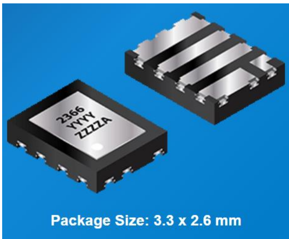
Figure. The 40-V, 0.8-m \Omega GaN FET offers an R_{ON} \times Q_G figure of merit (10 m \Omega nC), which is best-in-class according to the vendor. The company has also announced plans to introduce 25-V and 15-V GaN devices.
