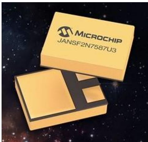
Figure. The JANS series of rad-hard power devices is available in voltage ranges from 100 V to 250 V and TID to 100 Krad (Si), with the family expanding to higher RHA levels, starting with the JANSF2N7587U3 at 300 Krad (Si) TID.
