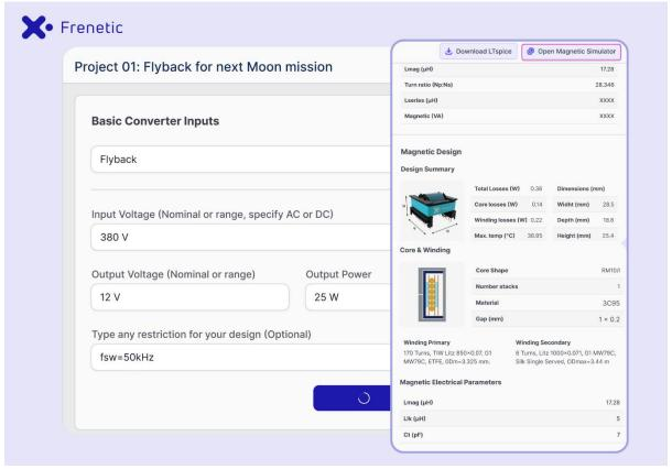
Figure. With Frenetic AI, users enter electrical specs for their power supply project. The tool can then either search for an off-the-shelf power supply, or suggest a power supply topology. In the latter case, Frenetic AI will create the power supply design, automatically generating a schematic, BOM, and simulation files, and then running simulations. The simulation files are LTspice or PLECS. Frenetic AI also suggests suitable off-the-shelf or custom magnetics.
