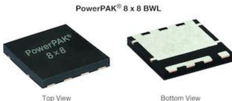
Figure. Housed in the PowerPAK 8x8SW bond-wireless package, the SiEH4800EW n-channel 80-V MOSFET is a space-saving device offering a max R_{TH(JC)} of just 0.36°C/W and wettable flanks to improve thermal performance and solderability in industrial applications.
