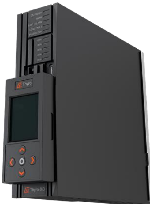
Fig. 1. Measuring 46 mm (w) x 150 mm (h) x 154 mm and weighing 0.9 kg, the Thyro-XD digital thyristor SCR power controller is compact, lightweight and easy to connect to process and automation technology. With a high accuracy of <0.5% it is well suited for highly dynamic applications. The power controller targets SEMI lamp driver processes such as epitaxial growth and rapid thermal annealing applications.
