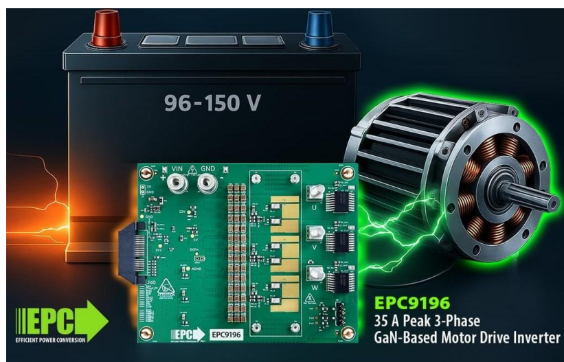
Fig. 1. The EPC9196 is a 25-Arms, three-phase BLDC motor drive inverter design optimized for 96-V to 150-V battery applications such as those found in robotics, automated guided vehicles (AGVs), and compact EVs. It leverages the low losses of the EPC2304, a 200-V-rated, 3.5-m \Omega (typical) eGaN FET in a thermally enhanced QFN package.
