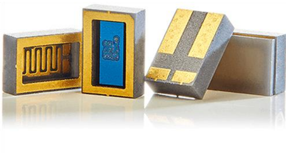
Figure. The EPC7030MSH is a 300-V, 35-m \Omega rad-hard eGaN FET in a surface-mount FSMD-M hermetic package.
