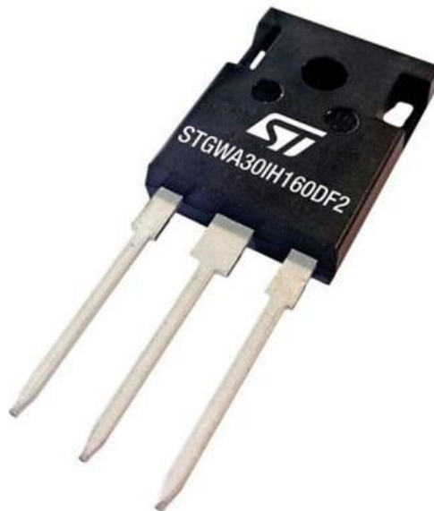
Figure. The STGWA30IH160DF2 is the first 1600-V IGBT in ST's IH2-generation. The IH2 series has been developed using an advanced proprietary trench gate field-stop structure, whose performance is optimized both in conduction and switching losses for soft commutation. A freewheeling diode with a low drop forward voltage is included. The result is a product specifically designed to maximize efficiency for any resonant and soft-switching applications.
