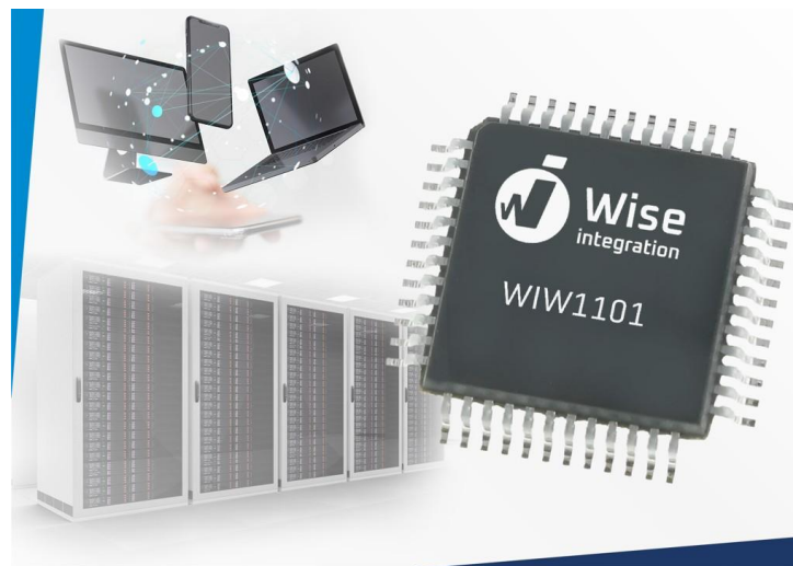
Figure. Unlike legacy analog solutions, WiseWare 1.1 leverages the speed and switching capabilities of GaN through a proprietary digital control algorithm in a 32-bit MCU, which enables zero voltage switching across all power transistors. Designed specifically for totem pole power-factor correction (PFC) architectures in critical-conduction mode (CrCM), this controller allows engineers to dramatically reduce the size, weight, and thickness of magnetic components while maintaining >98% efficiency.
