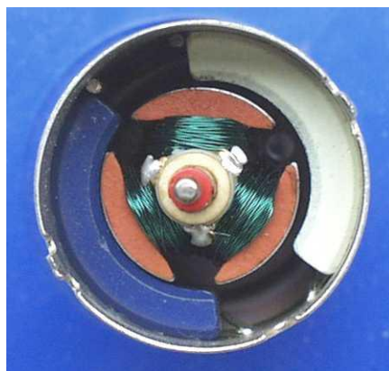
Fig. 3. A Mabuchi RE-36 motor with end-bearing removed (for photo). The windings are brought out the other end and the stator and shaft made stationary while the magnets and case, comprise an outer rotor. (Movement range is less than one mechanical revolution because of the wire access window in the rear-bearing plate.)
