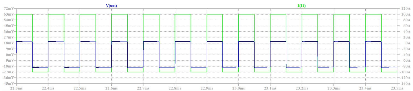
Fig. 3. Timing diagram of the Rogowski sensor operation. Shown here are the measured current waveform (green trace) and the sensor output voltage (dark blue trace).
