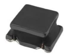
By filling the winding wire with resin containing magnetic material, the magnetic shield effect and the mechanical impact strength are significant. These low-profile components feature ferrite core construction and operate over a temperature range of -40°C to 125°C including the coil's temperature rise.
