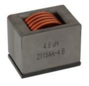
The edge-wound coil of the devices provides low DCR down to  $0.22~m\Omega$ , which minimizes losses and improves rated current performance for increased efficiency. Compared to competing ferrite-based solutions, they offer 30% higher rated current and 30% higher saturation current levels at +125°C. The inductors' soft saturation provides a predictable inductance decrease with increasing current, independent of temperature.
