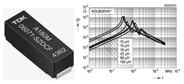
A power injection choke, the ADL8030VA measures 7.8-  $\times$  2.7-  $\times$  2.7-mm and features high impedance over frequency.
