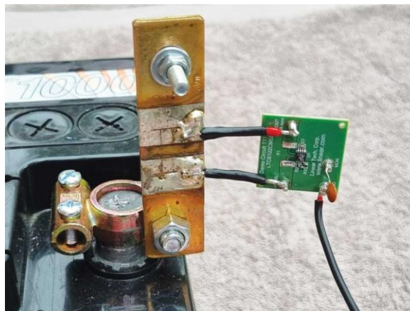
Fig. 9. The complete current sense circuit for measuring the battery current. The demo board for the LTC6102 (25 mm x 25 mm) illustrates the small size of the sensing circuit.
