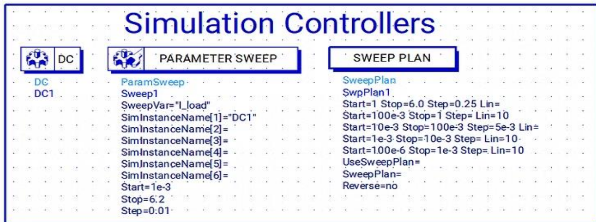
Fig. 2. Keysight ADS dc simulation setup with parameter sweep and sweep plan.
