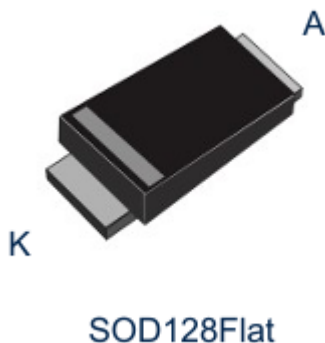
Figure. Manufactured using ST's space-proven power Schottky and ultrafast technologies, the LEO1N58xx family meets the new space industry's stringent demands for cost-effectiveness, radiation hardness, small size, quality assurance, and higher-volume availability, says the vendor. The LEO1N5819 and LEO1N5822 Schottky diodes offer 1-A , 45-V and 3-A, 40-V performance respectively, while the ultra-fast LEO1N5811 operates at up to 6 A and 150 V.
