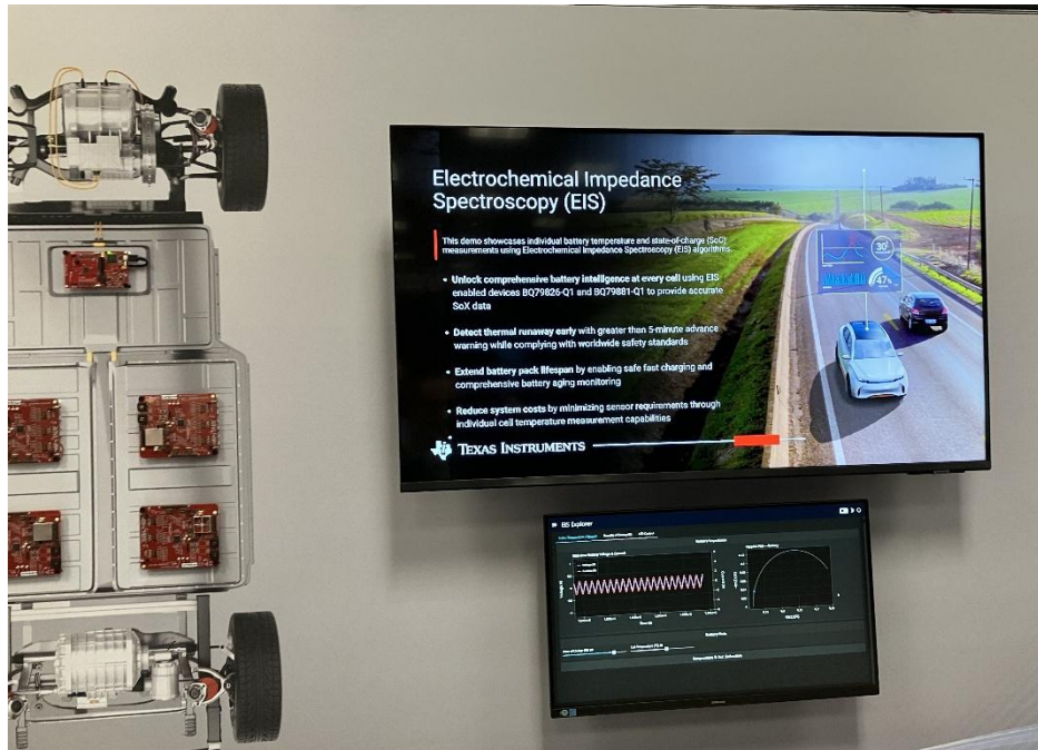
Fig. 5. TI’s demos included a wireless BMS (pictured on the left) and EIS-based battery measurements (pictured on the right). By monitoring battery conditions at the cell level, EIS measurements and algorithms enable early detection of pending thermal runaway events, and more comprehensive monitor of battery aging. This capability prevents fires, enabling faster charging and extending operating life of battery packs in EVs and energy storage systems.
