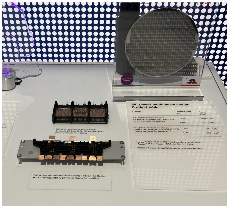
Fig. 2. Bosch's exhibit on its Smart SiC power semiconductor portfolio displayed Gen 2 of the company's bare die SiC MOSFETs, which feature improved R_{DS(on)} * Area FOM, short circuit robustness and capacitance; the company's packaged discrete SiC MOSFETs and its SiC power modules-on-cooler products.
