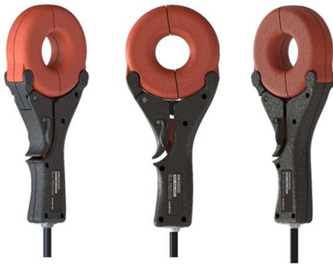
Fig. 1. With the introduction of the MK500ID, the company offers its first current transducer in the clamp-on style. It also features very high bandwidth (1 MHz), a phase shift of just 0.05^\circ at frequencies below 100 Hz and high linearity (20 ppm).
