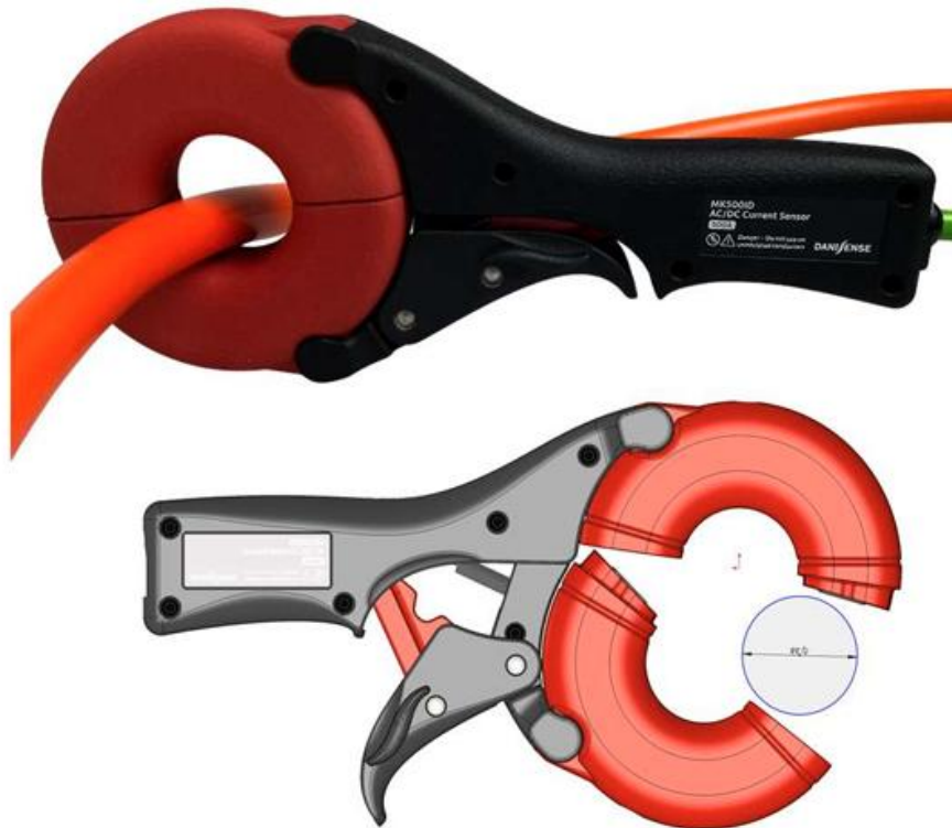
Fig. 2. The MK500ID employs a vertical translation mechanism that allows the customer to use the full diameter of the hole, allowing it to accommodate cable diameters up to 39 mm. Conveniently, it's also designed for one-hand operation.
