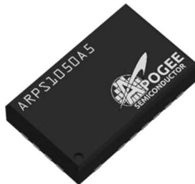
Figure. The ARPS1020A5 and ARPS1050A5 are radiation-hardened-by-design power switches with integrated FET. The 50-V variant supports the 28-V nominal bus voltage typically found in power distribution systems of a spacecraft, while the 20-V variant is well suited for a 12-V bus or at lower voltage loads such as 5 V and 3 V.
