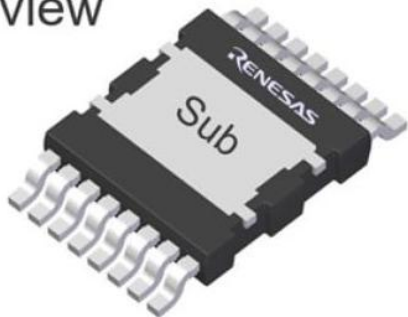
Figure. Targeting single-stage solar microinverters, AI data centers and onboard electric vehicle chargers, the TP65B110HRU 650-V 110-m \Omega bidirectional power switch is said to dramatically simplify power converter designs by replacing conventional back-to-back FET switches with a single low-loss, fast-switching, easy-to-drive device. Housed in a top-side cooled TOLT, the device co-packages the d-mode GaN chip with two low-voltage silicon MOSFETs.
